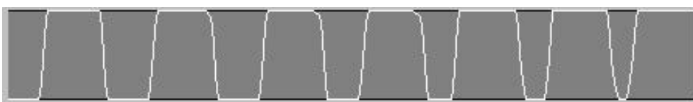
Figure 24 – Waveform with gain too high
